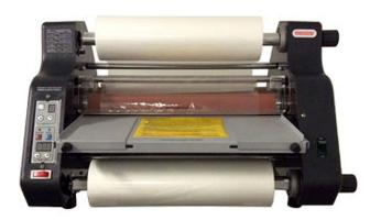
The **TCC-1400i** is a **14"** professional grade roll laminator for volume laminating of documents less than 14" wide. This heated roller laminator is capable of laminating up to 10mil in thickness and mounting up to 3/16" board.
