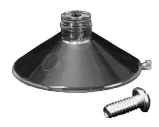
This medium-sized suction cup has a 1/8" stem hole. It is furnished with a 1/8-inch diameter x 1/2-inch long pan head screw. The screw fits the suction cup's stem hole and is used to affix signs to the suction cup.
