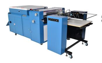
The **Spectra-Coat 25" UV Coater** is available as a hand-fed unit or with an air feeder. A deep-pile outfeed stacker is also available. It runs up to one-quarter inch thick substrates, with an option of running up to 1 inch thick substrates.
