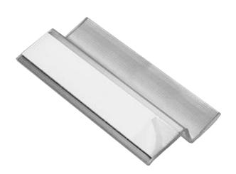
**Slat wall clips** hold lightweight signs to slat walls. Peel-and-stick foam tape attaches the sign to the clip. Positioning the sign is as easy as sliding it back and forth in the slat.
