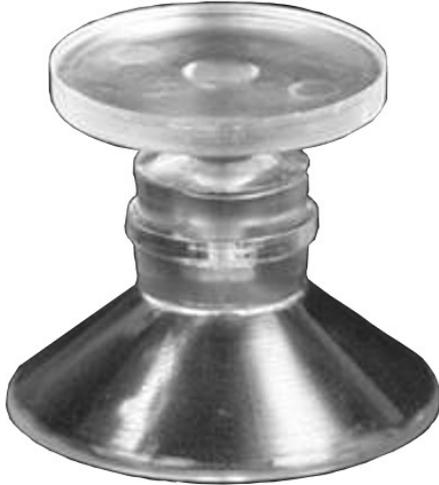
These suction cups have a hole in the stem that accepts a clear tack. The tack pierces sign stock, or passes through drilled or punched holes. It then grips the corresponding hole in the suction cup's stem, holding your sign in place.
