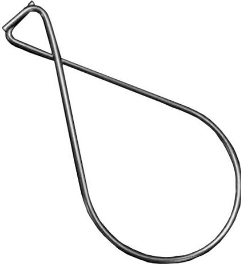
**Metal figure-8 clips** are an economical means of hanging light signs from grid ceilings. The clips squeeze open and grip ceiling grids when released. These simple, versatile clips are easy to install, remove, and reposition.
