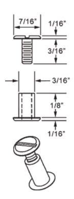
These 1/8" Aluminum Screw Posts come in packs of 100 sets. One set is one Screw and one Post.
