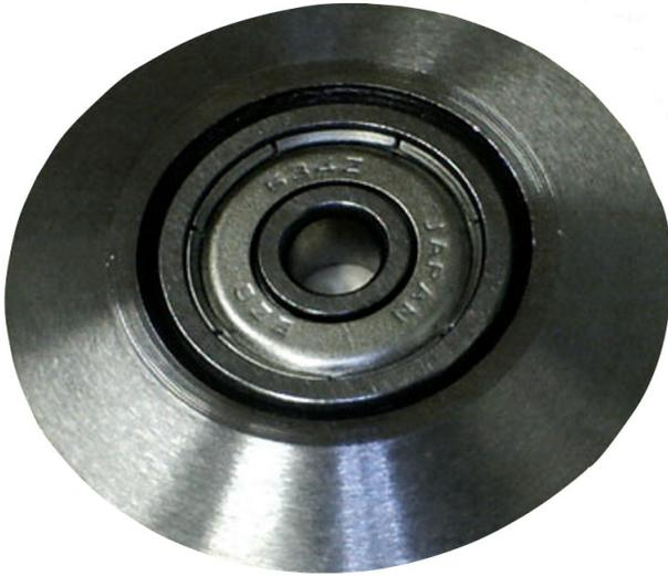
Replacement slitting blade for the Count machines that are capable of slitting.
