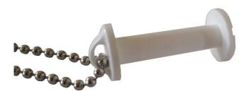
Loop screws with 3/8" binding capacity. They fit in 1/4" holes.
