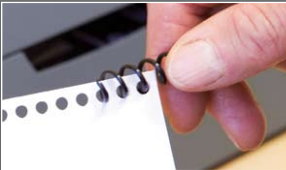
Start coil into the first three holes by hand.
